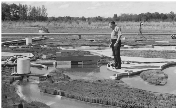
FIGURE 8 Mississippi River Basin Model with which engineers predict- ed floods 1943-1993. Source: https://99percentinvisible.org/episode/america-last-top-model (Accessed: 3 November 2017)
